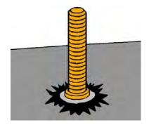
A one sided stud weld (arc blow) is usually caused by incorrect earthing of the work piece. This may be corrected by placing the welding earths opposite each other across the area where the weld is to occur.
