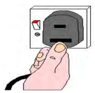
Connect the welding earth cables to the controller socket marked +. Note that the cable end plug has a peg which mates with a key slot in the panel mounted socket.
