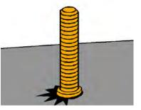
Finished studs may be subjected to a bending test to ascertain the strength of the weld. This may be achieved by placing a bending bar assembly, fitted with the correct nozzle, over the stud and bending the stud through 30° and then back to the vertical. This test follows the specification of BS EN ISO 13918.
