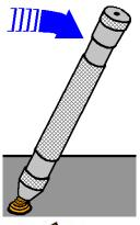
A simpler test may be achieved by bending the stud over 30° using a hide mallet.
