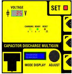
Within 5 seconds the MODE display will change to "Welding Mode" and the VOLTAGE display will change to match the voltage shown in the
