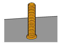
A hot stud weld is noticeable by excessive spatter formation and partial melting of the flange. A hot weld is usually by too much energy and / or too little spring pressure.
