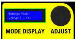
Repeat these two steps to set Voltages 2 & 3. After setting Voltage 3, press and release the "SET" button one more time. The MODE display will return to "Welding Mode Voltage = XX" (XX will now be the lowest number of the three voltages that have been pre-set above) and the VOLTAGE display will also show this value.
