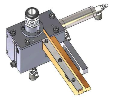
There are 2 stud sensors. The top one turns the bowl feeder on and off depending on whether it is covered or uncovered. If the bottom is uncovered it stops the system from welding.
