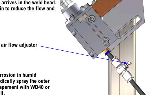
Note: To prevent corrosion in humid environments periodically spray the outer surfaces of the escapement with WD40 or similar protective oil.
